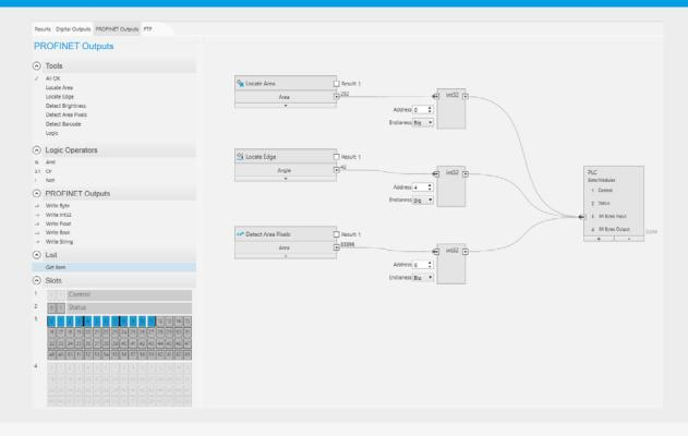
At the end of editing, the results can be summarized and transmitted to the higher-level control system using the options in the Logic area.
