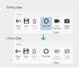
Select "Override" to execute a job. Now the sensor is active and ready to communicate with the higher-level control.
