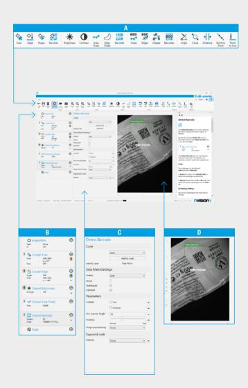
The CS-60 user interface is made up of 4 areas. The navigation bar in the upper area is for instructions and setup. The verification tools contained here are divided into 4 groups. Double-click on one of these tools to insert it in the area on the left, the so-called Pipeline. Configuration and parameterization of the selected tools can be performed in the area in the middle. Finally, on the right side there is an even larger field in which the image and the drawing tools are displayed.
