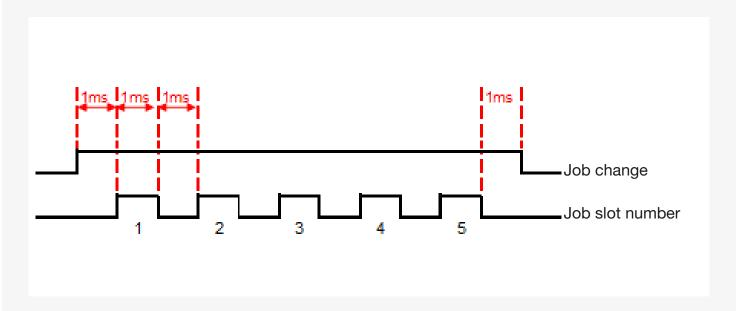
To do this, use the inputs 0 and 1. The PLC sets a high signal to the line 0 "Change job" and then sends a series of impulses (1 ms hold time) to line 1 "Job selection." The number of impulses then corresponds to the job number, e.g. 5 impulses = job number 5. After the 5th impulse and a wait time (Low side) of 2 ms, the signal to line 0 is then canceled (Low side).
